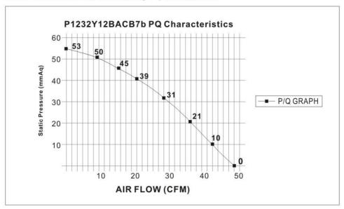
A. Calculate airflow through your system by applying the blower in your system and by measuring the incoming and outgoing airflow temperatures as follows:
